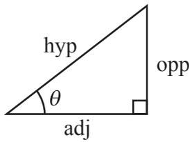
$$\begin{aligned} \text{adj} &= \text{hyp} \times \cos \theta \\ \text{opp} &= \text{hyp} \times \sin \theta \\ \text{opp} &= \text{adj} \times \tan \theta \end{aligned}$$
